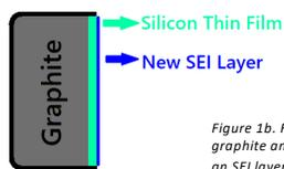
Figure 1b. Representative schematic of a graphite anode with a thin film of silicon and an SEI layer of a new composition distinct from 1a.
